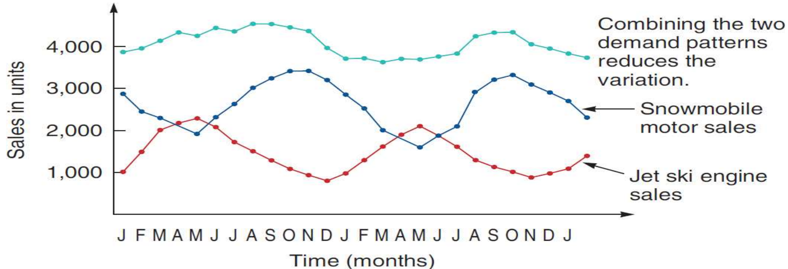
Figure S7.3 By Combining Products That Have Complementary Seasonal Patterns, Capacity Can Be Better Utilized
